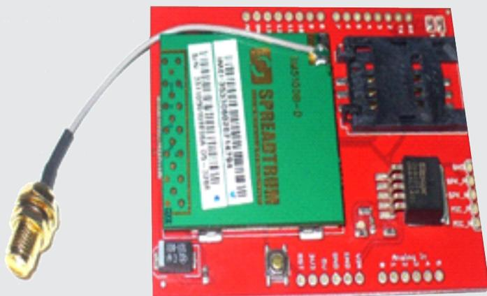
Figura 3. Tarjeta SM5100B Cellular Shield
