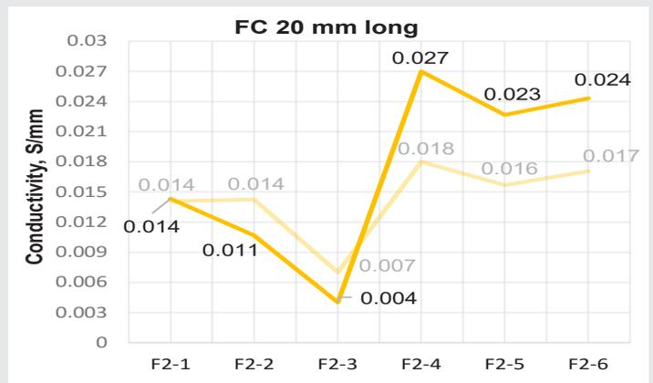
Graph 4. Conductivity of dry specimen with FC 20 mm long
